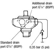
An additional drain port is provided when the "V" (shaft vertically upwards) designator is given after the shaft type letter in position **3** of the model code. This additional drain should be connected into the main motor casing drain line downstream of a 0,35 bar (5 psi) check valve to ensure lubrication of the upper bearing, see above diagram.
