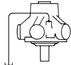
There are no special requirements for the drain line with this type of installation.
