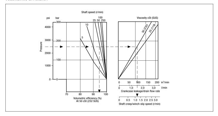
This nomograph enables the average volumetric efficiency, crankcase (drain) leakage and "winch slip"/shaft creep speed to be estimated.
