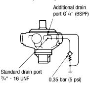
An additional G<sup>1</sup>/<sub>4</sub>" (BSPF) drain port is provided when the "V" (shaft vertically upwards) designator is given after the shaft type letter in position 3 of the model code. This additional drain should be connected into the main motor casing drain line downstream of a 0,35 bar (5 psi) check valve to ensure lubrication of the upper bearing, see above diagram.
