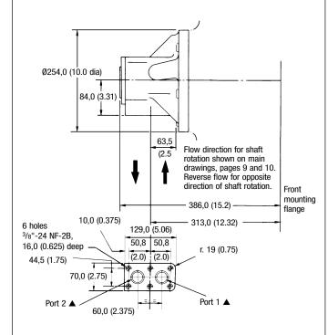
▲ Ø28 (1.125 dia) with recess for 31,0 (1.22) i/d x Ø 4 (0.57 dia) section 0-ring
