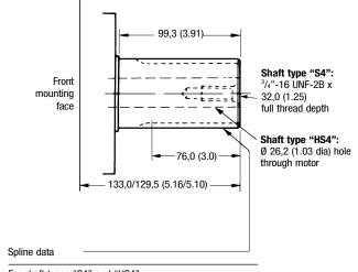
For shaft types "S4" and "HS4" Involute gear tooth form Pressure angle Number of teeth 16 Pitch 5/10 Major diameter 86,360/86,233 (3.400/3.395) Form diameter 76,124 (2.997) Minor diameter 74,93/72,39 (2.95/2.85) Pin diameter 8,636 (0.3400) Diameter over pins 92,71/92,581 (3.650/3.645)
