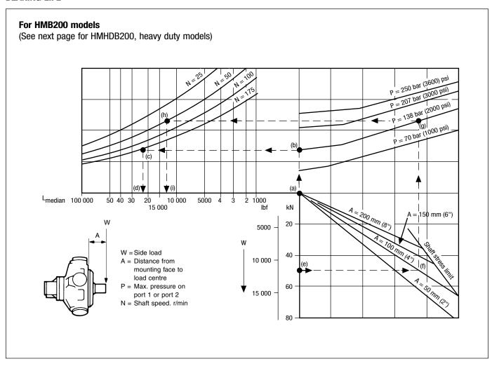
The nomographs on this and the following page allow the median bearing life to be determined for conditions of:
