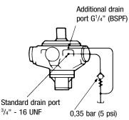
An additional G<sup>1</sup>/4" (BSPF) drain port is provided in the front cover when the "V" (shaft vertically upwards) designator is given after the shaft type letter in position **3** of the model code. This additional drain should be connected into the main motor casing drain line downstream of a 0,35 bar (5 psi) check valve to ensure lubrication of the upper bearing, see above diagram.
