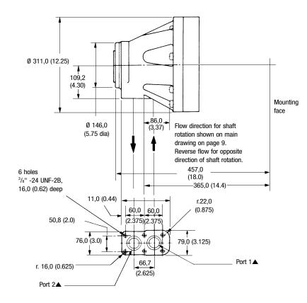
▲ Ø 35,0 (1.325 dia), with recess for 38,1 (1.5) i/d x Ø 3,53 (0.139 dia) section 0-ring
