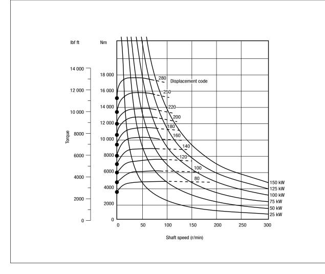
The torque curves indicate, for each displacement, the maximum output torque of the motor with an inlet pressure of 250 bar (3626 psi) and zero output pressure. High return line pressure will reduce the torque for any given pressure differential.
