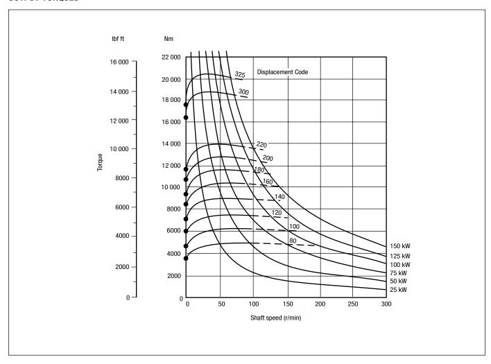
The torque curves indicate, for each displacement, the maximum output torque of the motor with an inlet pressure of 250 bar (3626 psi) and zero output pressure. High return line pressure will reduce the torque for any given pressure differential.
