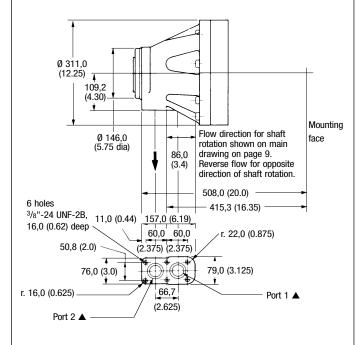
▲ Ø38,1 (1.5 dia), with recess for 38,1 (1.5) i/d x Ø 3,53 (0.139 dia) section 0-ring
