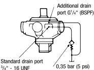
An additional G¹/4" (BSPF) drain port in the front cover is provided when the "V" (shaft vertically upwards) designator is given after the shaft type letter in position of the model code. This additional drain should be connected into the main motor casing drain line downstream of a 0,35 bar (5 psi) check valve to ensure lubrication of the upper bearing, see above diagram.
